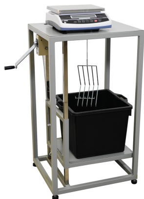
Specific gravity frame with electronic balance and cradle for specimens
